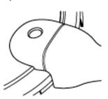
**PRESSURE REGULATOR** Controls and maintains pressure inside the cooker and indicates when the ideal cooking pressure - usually 15 pounds - is reached.
