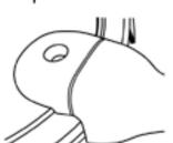
Air Vent/Cover lock in UP position indicates pressure in unit.
