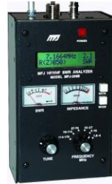
SWR Meter measures the standing wave ratio in a transmission line.
