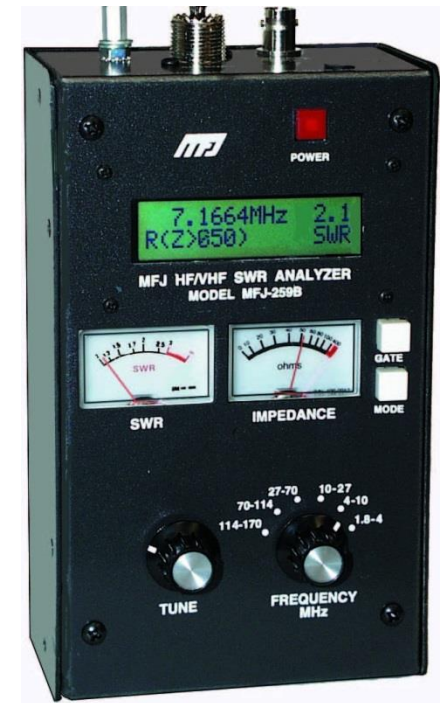
SWR Meter measures the standing wave ratio in a transmission line.
