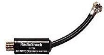
This high-pass filter goes between the TV and antenna
